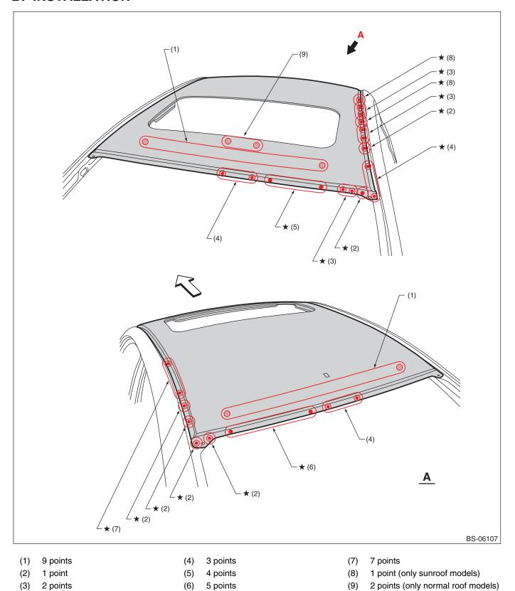
For locations marked by "★": the welding method and the number of welding points are the same on the left and the right.
